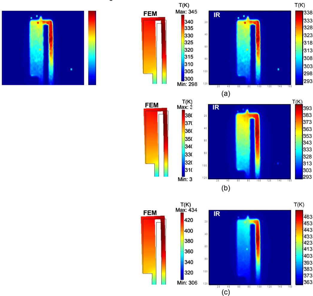
**Fig.2.** Comparison between IR measurements and FEM simulation results (a) 190mW input power, (b) 305mW input power, (c) 425mW input power
