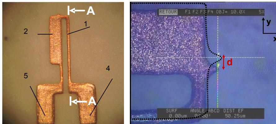
Fig 1 Measurement of actuator tip deflection  $d$ .
